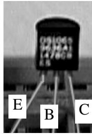
Photo of the 3904 BJT in the TO-92 plastic package. With the flat side facing you, the leads are, from left to right, Emitter, Base, Collector.
